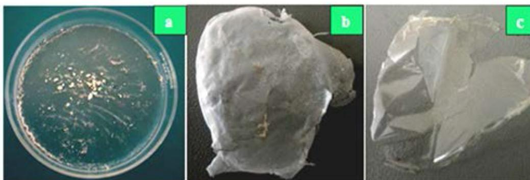
Figure 2: PHAs Polymer a) powder polymer extracted from bacterial isolate b) The neat biofilm sheet produced by chloroform method c) Modified form of the neat film blends using ethylene oxide.
