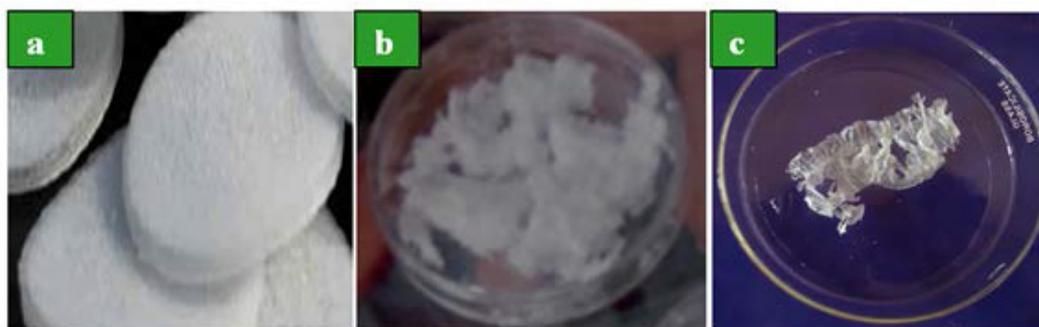
Figure 3: Examples of PHAs scaffolds fabricated for tissue engineering applications, a) Meshes b) Woven c) Fibers.
