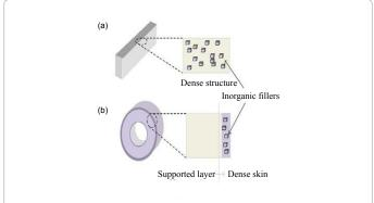
**Figure 1:** MMMs in configuration: (a) symmetric flat dense, and (b) Asymmetric hollow fiber [7].
