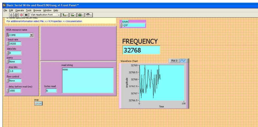
Figure 7: Front Panel of LabVIEW Program of PSoC embedded design for QTF for humidity measurement.
