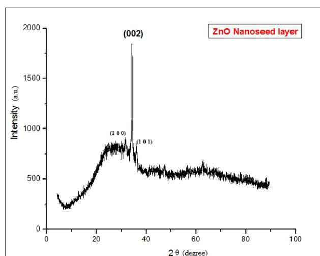
Figure 3: XRD pattern of SILAR grown ZnO nanostructure seed layer taken using PAN alytical (X'PERT-PRO) X-Ray diffractometer.
