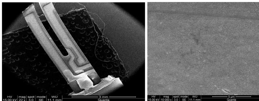
Figure 1: SEM picture of encapsulated QTF and uncoated QTF taken using ICON Analytical (FEI QUANTA 200) Scanning Electron Microscope.
