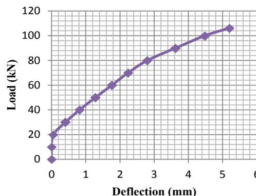
Figure 5: Load deflection curve for retrofitted beam with 30% addition of Alccofine.
