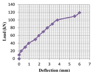
Figure 3: Load deflection curve for retrofitted beam with 10% addition of Alccofine.
