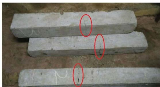
Figure 6: Crack pattern of retrofitted concrete beams.
