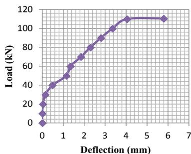
Figure 2: Load deflection curve for retrofitted beam with cement mortar.
