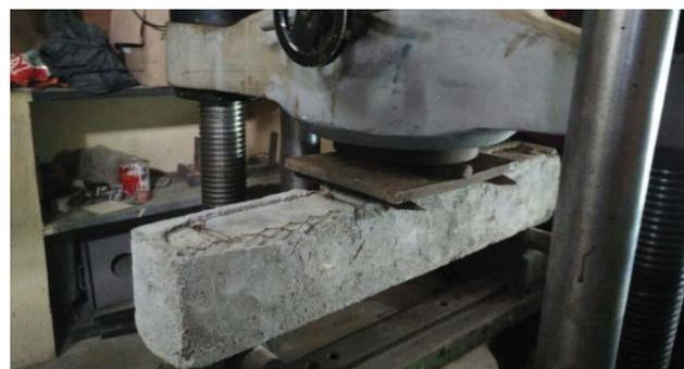
Figure 1: Flexural testing of retrofitted RC beams specimen.
