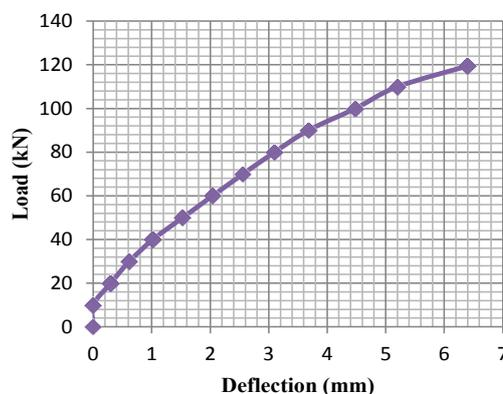
Figure 4: Load deflection curve for retrofitted beam with 20% addition of Alccofine.
