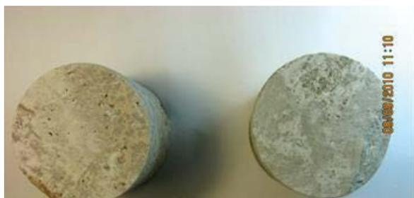
**Figure 5:** At the left a fragment of core B after acid treatments in the laboratory; at the right a fragment of core D as it is, without any acid treatment in the laboratory.
