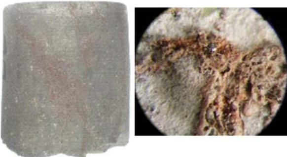
**Figure 3:** At the left a piece of the untreated core B (15 cm x 8 cm). At the right an image of a fragment of core B after reaction with the binary acid mixture, (16X).
