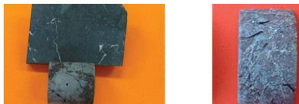
**Figure 2:** Core A. At the left, on top, the original fragment of the core A, below it after HCl treatment; at the right the same fragment after reaction in HCl+HF solution. Open conduits and rough surface are observed. Dimension of specimens are 3.5 cm in diameter and 3-4 cm high.
