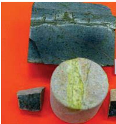
**Figure 4:** A fragment of core C, before acid treatment, with a vein sealed by quartz and epidote. After reaction in acid solutions the cylinder shows a bleached surface and no dissolution of quartz and epidote. The size of the cylinder is 3.5 cm of diameter and 4 cm height.
