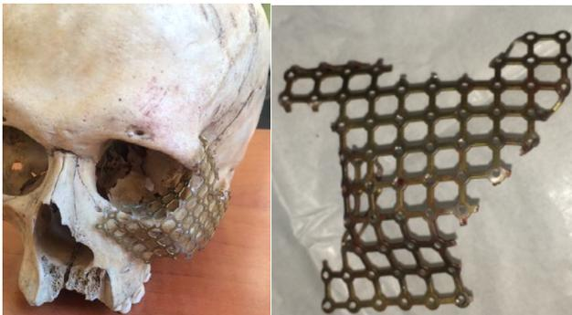
Figure 3: Titanium mesh adaptation: (a) adaptation on the phantom skull, (b) finally suited mesh.
