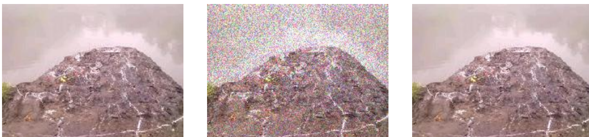
Fig. 6 a) Original SAR Image b) Degraded SAR Image by Speckle noise with variance 0.04 c) Denoised SAR Image
