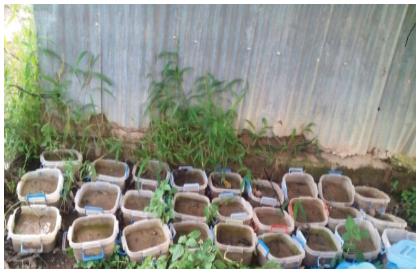
Figure 5: Experimental setup of bioremediation (27 field cells).
