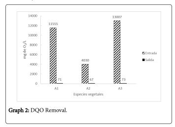
In Graph 2, it can be seen that in the three days of analysis, COD values were obtained at the inlet of 11555 mg/l, 4030 mg/l and 13007 mg/L, and values of 71 mg/L were recorded at the outlet. 67 mg/L and
