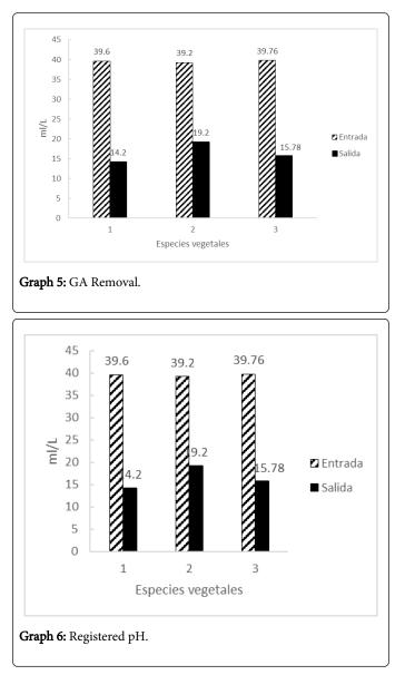
As can it be seen in Graph 6, the pH, both, at the entrance and at the exit, along the three days of the study, it does not show significant changes, presenting a minimum value of 6.72 at the entrance and 6.52 at the exit; and maximum values of 7.11 at the entrance and 6.62 at the output.
