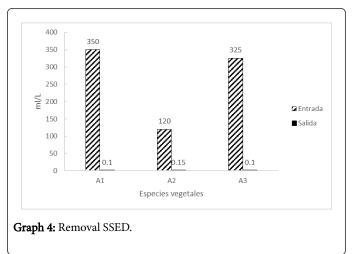
Graph 4 shows the SSED values contained in the water, which are 350 ml/L, 120 ml/L and 325 ml/L, and at the outlet of 0.1 ml/L, 0.15 ml/L and 0.1 ml/L; indicating a removal, of almost 100% of solids sedimentables (Graph 5).
