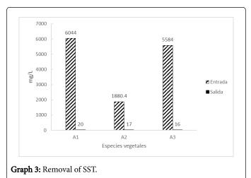
For the SST parameter, in Graph 3 the obtained values are recorded, in the input there were 6044 mg/l, 1880.4 mg/L and 5584 mg/L; and at the outlet of 20 mg/l, 17 mg/L and 16 mg/L, obtaining, removal percentages above 99%.
