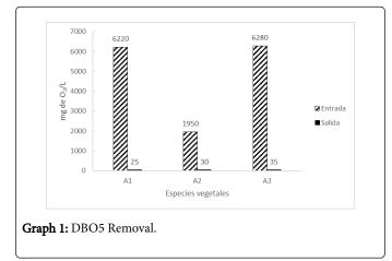
As it can be seen in Graph 1, the BOD5 at the entrance reached values of 6280 mg  $O_2/L$ , 6220 mg  $O_2/L$  and 1950 mg  $O_2/L$ ; at the exit, after having had removals between 98% and 99%, values of 25, 30 and 35 mg  $O_2/L$  were recorded, demonstrating the high efficiency of the treatment system.
