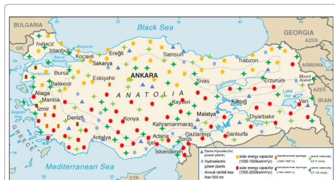
Figure 7: Distribution of hydro power, solar energy, geothermal fields having temperatures greater than 100°C and wind energy potential in Turkey.
