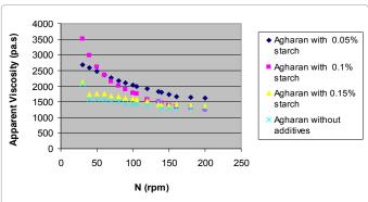
Figure 9: Apparent viscosity versus N for different concentration of Agharan contains Starch.
