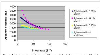
Figure 3: Apparent viscosity versus Shrear rate for Agharan contains different concentration of Starch.
