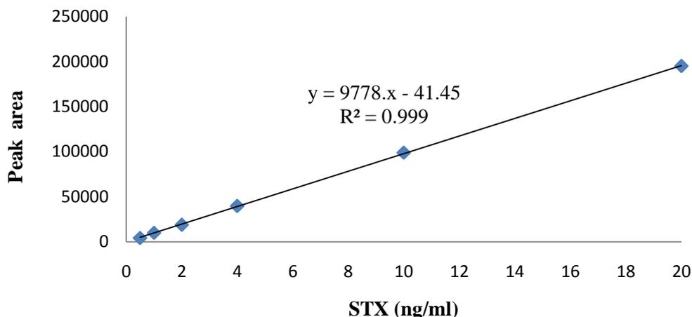
**Fig. 2.** Calibration curve of STX standard at concentration of 0.5-20ng/ml
