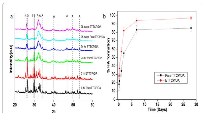
**Figure 2:** (a) XRD patterns of the cement and (b) percentage HA formation in the cement immersed in PBS at various time intervals (A=HA, T=TTCP and D=DA).
