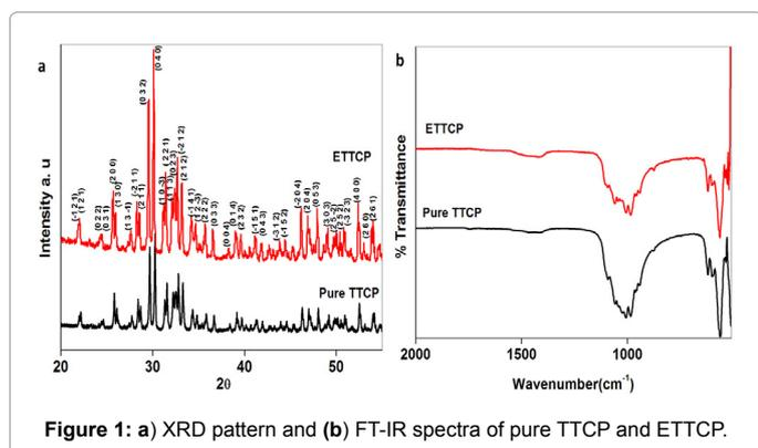
Figure 1: a) XRD pattern and (b) FT-IR spectra of pure TTCP and ETTCP.
