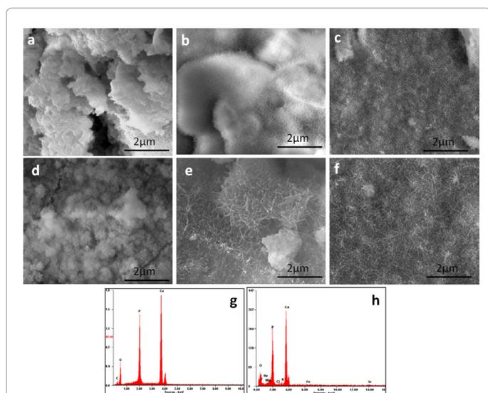
**Figure 3:** SEM image of the fractured surface of cement sample immersed in PBS. a, b and c correspond to the pure TTCP/DA and d, e and f correspond to the ETTCP/DA at 24 h, 72 h and 1 week respectively. g and h corresponds to the EDS spectrum of c and f respectively.
