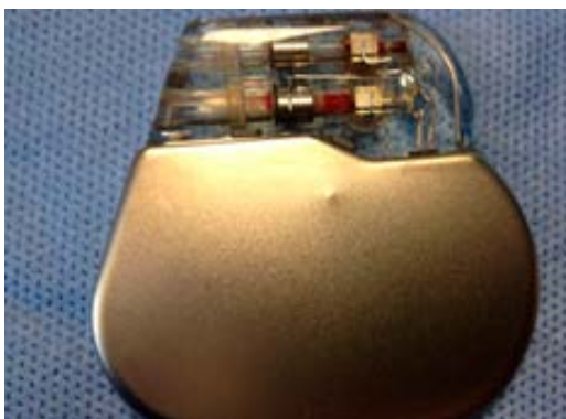
Figure 3: Rear view of can post explant Arrow indicates protrusion from impact through pulse generator.
