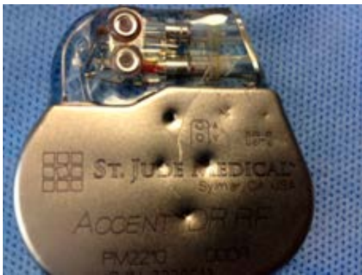
Figure 2: Front view of can post explant. Arrows indicate penetration of titanium Pulse generator case.
