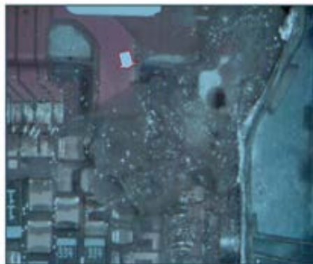
Figure 5: Opened can with body fluids inside of titanium case and noted on the hybrid.
