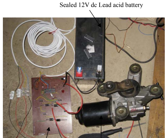
Vero board with all components soldered
