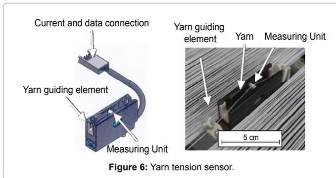
Figure 6: Yarn tension sensor.
