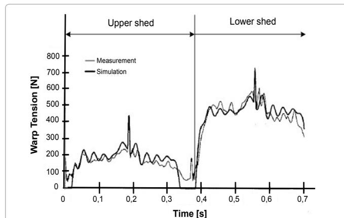
Figure 1: Comparisons of warp tension measurement and simulation by De Weldige [4].
