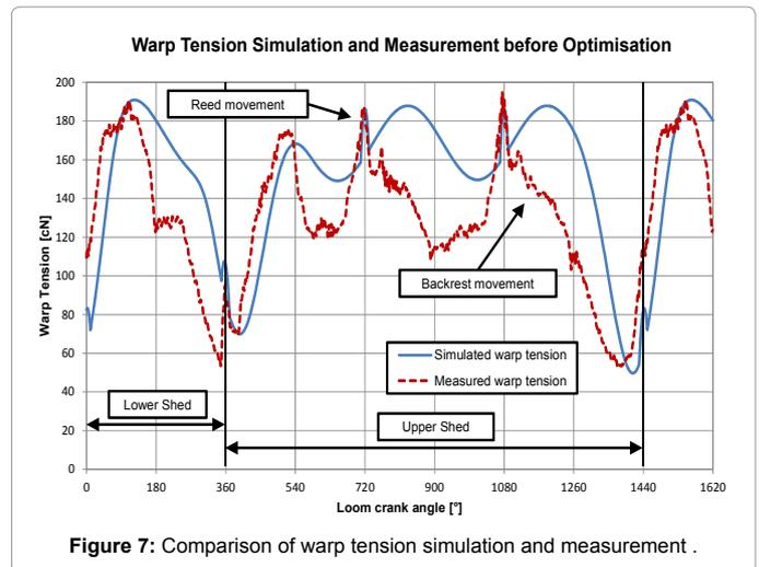
Figure 7: Comparison of warp tension simulation and measurement .
