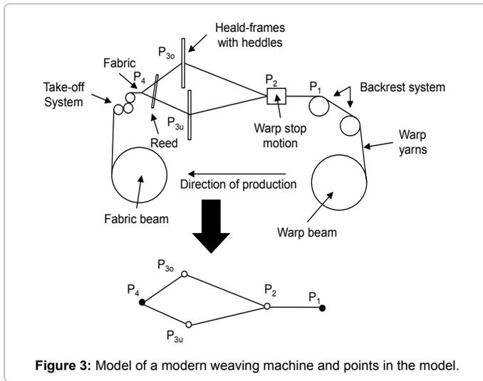
Figure 3: Model of a modern weaving machine and points in the model.
