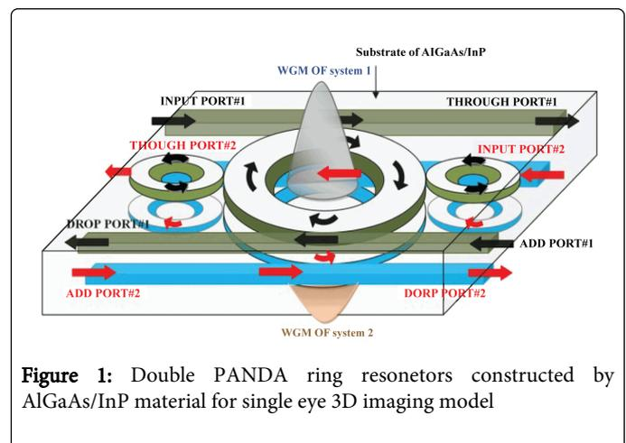
**Figure 1:** Double PANDA ring resonators constructed by AlGaAs/InP material for single eye 3D imaging model
