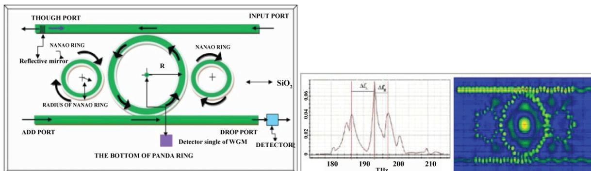
Figure 2b: Two micro conjugate mirrors using using AlGaAs/InP materials, where (b) Bottom ring with four waves mixing signals (bottom figure)
