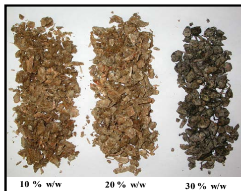
Figure 14: Shrimp shells after 144 h of deproteinization as affected by the initial galactose concentrations.
