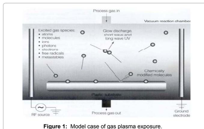
Figure 1: Model case of gas plasma exposure.
