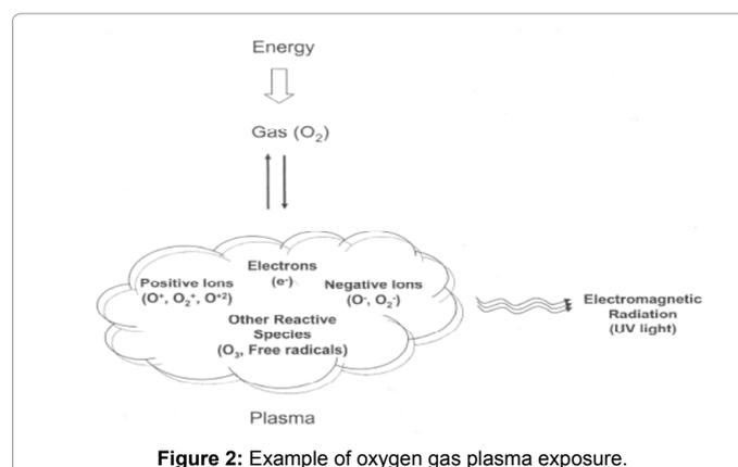
Figure 2: Example of oxygen gas plasma exposure.
