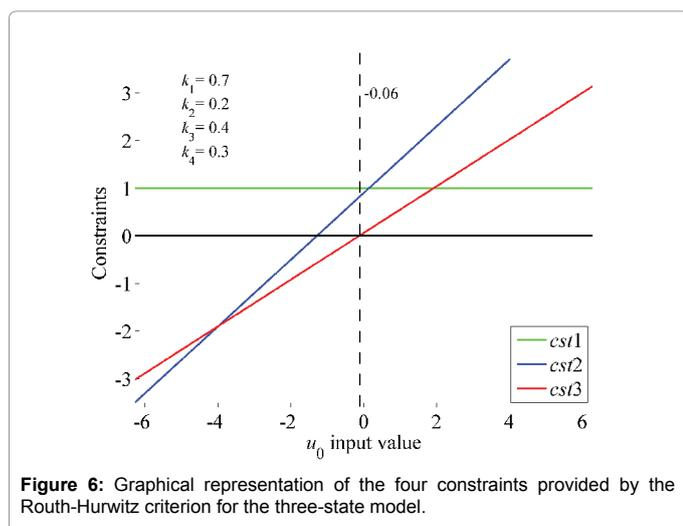
Figure 6: Graphical representation of the four constraints provided by the Routh-Hurwitz criterion for the three-state model.
