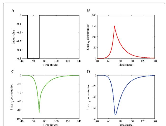
**Figure 5:** Simulation of the simplified model, using parameter values that do not satisfy stability constraints. A: input of the system. B: state  $x_1$ . C: state  $x_2$ . D: state  $x_3$ . States  $x_2$  and  $x_3$  are unstable as there are negative.
