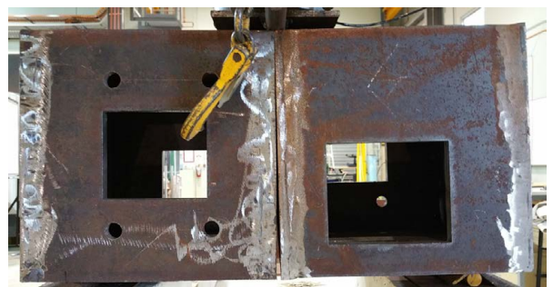
Figure 12: Observed gap between two brackets (7.89 mm) at 600 kN loading.
