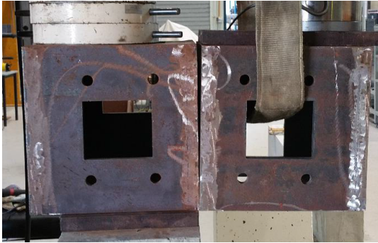
Figure 9: Specimen 2 - Deformed shape after failure load (414.0kN).
