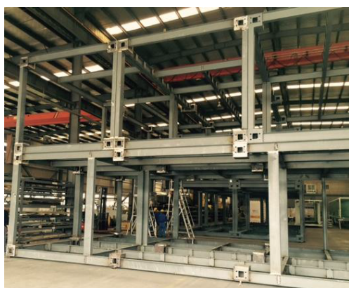
Figure 2: Steel connection assembled in a warehouse.
