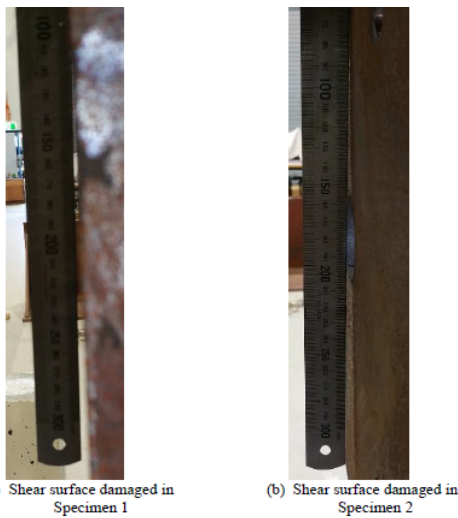
Figure 10: Deformed shear surfaces.
