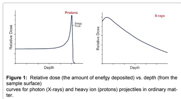
**Figure 1:** Relative dose (the amount of energy deposited) vs. depth (from the sample surface) curves for photon (X-rays) and heavy ion (protons) projectiles in ordinary matter.
