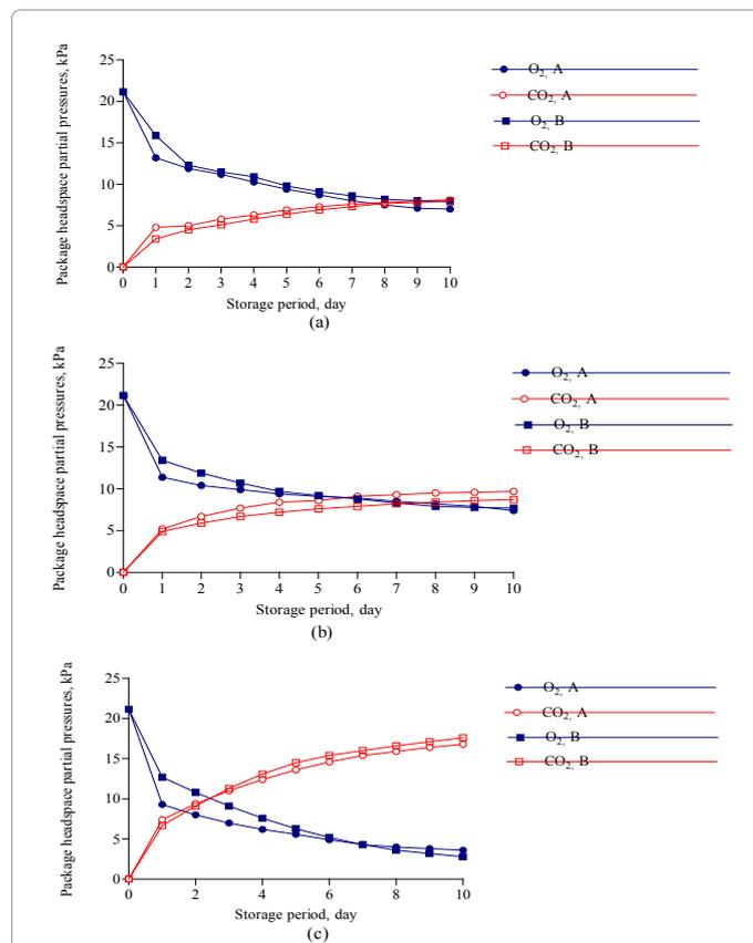
**Figure 4:** Headspace partial pressures of O<sub>2</sub> and CO<sub>2</sub> inside low density polyethylene (LDPE) film packages having different perforations (A: without perforations, B: 2 perforations) at (a) 5°C, (b) 12.5°C, (c) 20°C, kept for storage under modified atmospheres. The plotted values are means of headspace measurements per packaging treatment along with their standard deviations.
