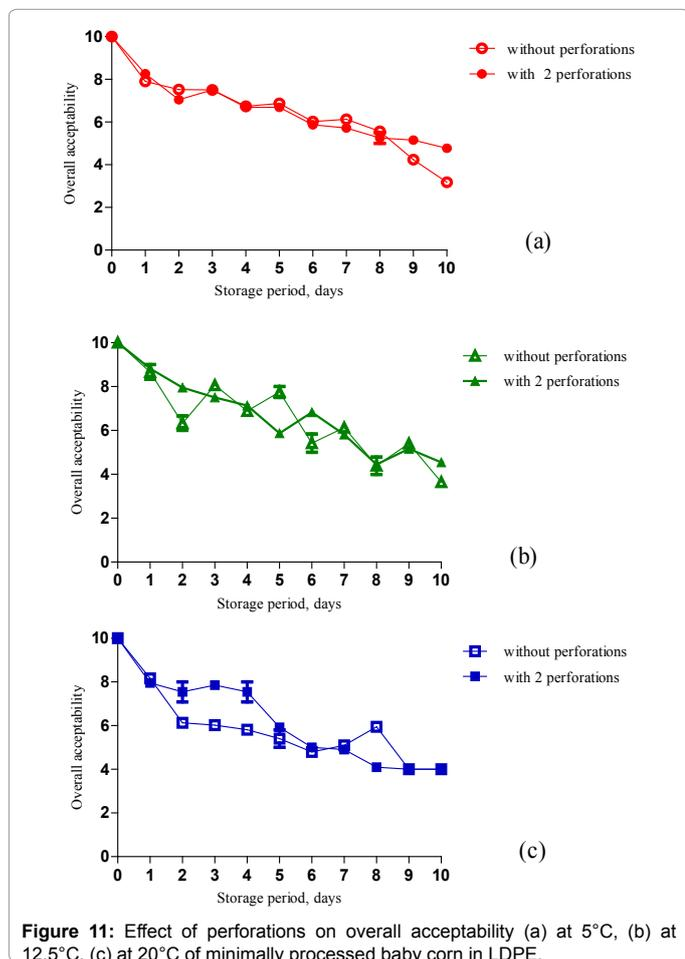
**Figure 11:** Effect of perforations on overall acceptability (a) at 5°C, (b) at 12.5°C, (c) at 20°C of minimally processed baby corn in LDPE.
