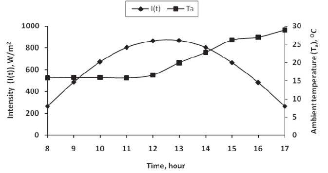
**Figure 1:** Hourly variation of solar intensity and ambient temperature of a typical day in the month of March.
