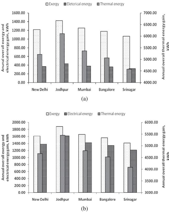
**Figure 2:** (a) Annual gain in overall thermal energy, exergy, and electrical energy for five different cities of India for case A ( $N = 3$  and  $T_{fo} = 40^\circ\text{C}$ ). (b) Annual gain in overall thermal energy, exergy, and electrical energy for five different cities of India for case B ( $N = 3$  and  $T_{fo} = 40^\circ\text{C}$ ).
