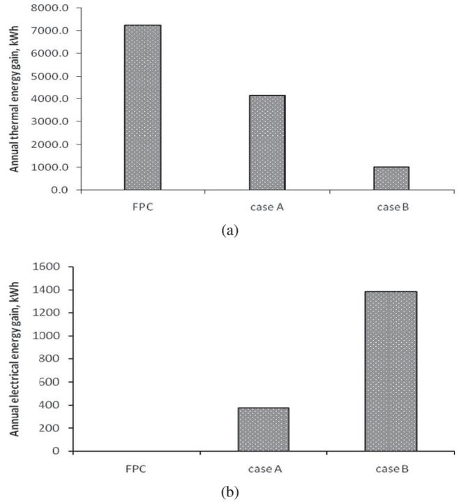
**Figure 3:** (a) Variation of annual thermal energy gain for FPC, case A, and case B for New Delhi weather conditions ( $N = 3$  and  $T_{fo} = 40^\circ\text{C}$ ). (b) Variation of annual electrical energy gain for FPC, case A, and case B for New Delhi weather conditions ( $N = 3$  and  $T_{fo} = 40^\circ\text{C}$ ).
