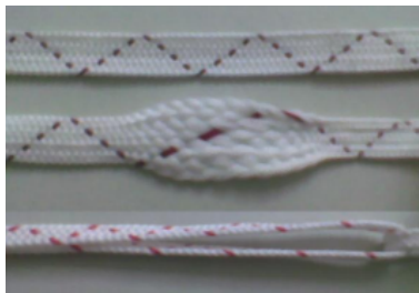
Figure 2: Different braided ACL types produced; flat (top), three-zone (middle) and double-band (bottom) ACL.
