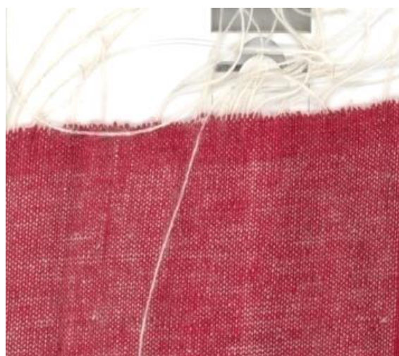
Figure 5: Sample II: Communication Fabric with Warp as 2/60s Ne Cotton and Weft as CK-20 POF.
