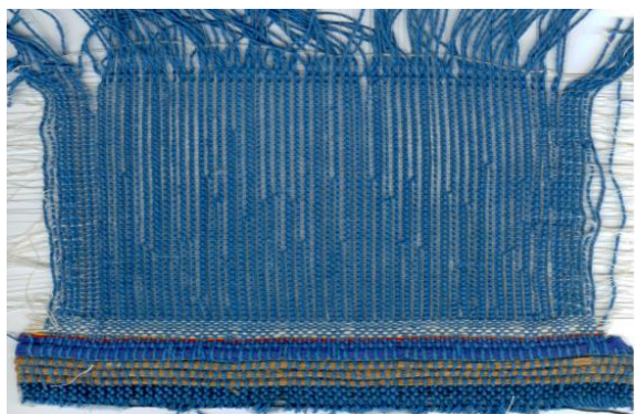
Figure 7: POF Integrated Fabric Using Power Loom.
