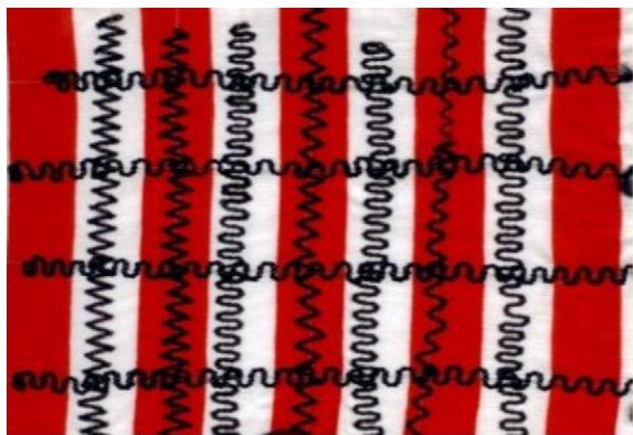
Figure 6: Integration POF in X-Y Direction on the Fabric.
