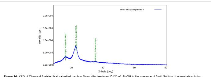
Figure 2d: XRD of Chemical Assisted Natural retted bamboo fibres after treatment **D** [20 g/L NaOH in the presence of 5 g/L Sodium tri phosphate solution  $(Na_5P_3O_{10})$ ].
