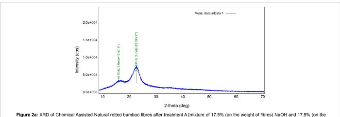
Figure 2a: XRD of Chemical Assisted Natural retted bamboo fibres after treatment A [mixture of 17.5% (on the weight of fibres) NaOH and 17.5% (on the weight of fibres) KOH.
