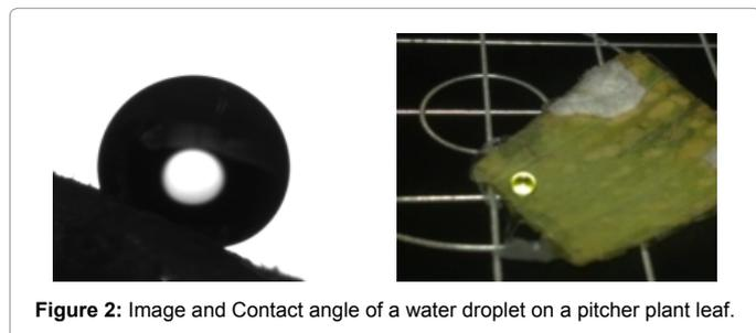
Figure 2: Image and Contact angle of a water droplet on a pitcher plant leaf.
