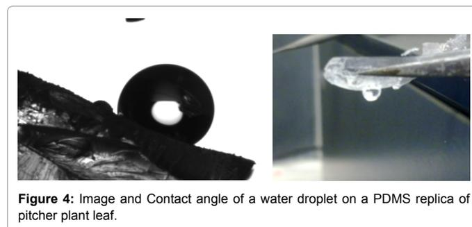
Figure 4: Image and Contact angle of a water droplet on a PDMS replica of pitcher plant leaf.
