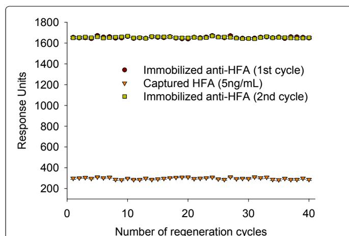
**Figure 3:** Reproducibility of antibody immobilization and antigen detection on the SPR Au chip, which was reused 40 times after regenerating the Au surface using the developed procedure. This process was mainly cycles of surface functionalization, assay performance, and regenerating the surface followed by repeating the cycle over 40 times. Error bars are %CV.
