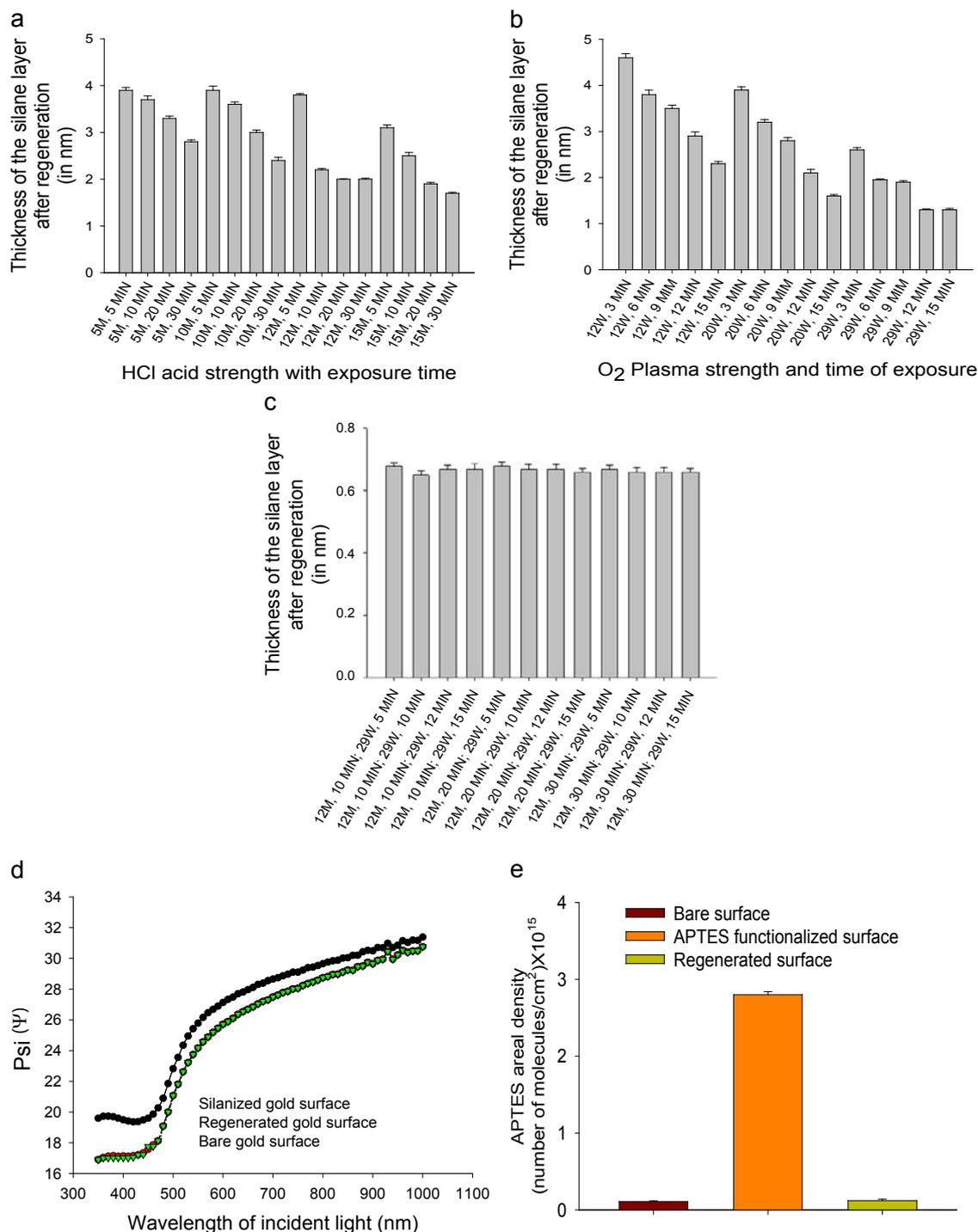
**Figure 2:** Optimization of surface regeneration procedure (a) siloxane bond lysis at various acid (HCl), (b) various O<sub>2</sub> plasma, and (c) their combined strengths as a function of exposure time (min). Thickness for each set was monitored using ellipsometry as depicted in 'd'. (e) Evaluation of areal density of APTES on bare, APTES-functionalized and regenerated Au surfaces by Rutherford back scattering (RBS). Error bars are standard deviation.
