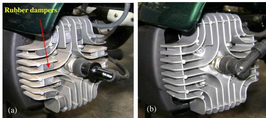
**Figure 1:** (a) Old engine with rubber dampers, (b) new engine without rubber dampers.
