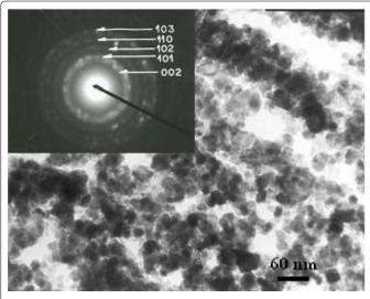
Figure 5: TEM images and electron diffraction patterns of ZnO nanoparticles at different temperatures.
