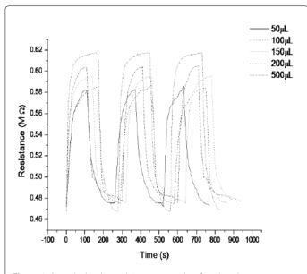
Figure 4: A graph showing resistance versus time for ethanol vapour sensors.
