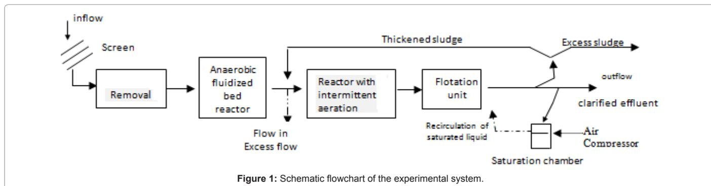
Figure 1: Schematic flowchart of the experimental system.
