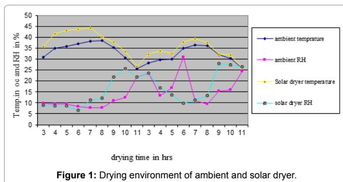
Figure 1: Drying environment of ambient and solar dryer.
