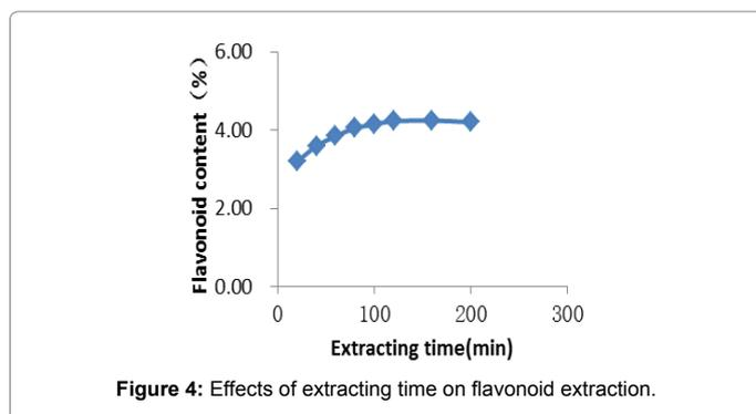
Figure 4: Effects of extracting time on flavonoid extraction.
