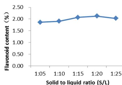
Figure 2: Effects of solid to liquid ratio on flavonoid extraction.
