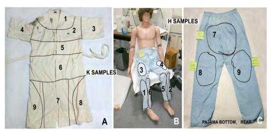
Figure 7: SEM sampler series H and K. Sixty dabs per sample. A: Sample regions of the bathrobe (samples K-1 through K-9). B: The front areas of the pajama bottom (Samples H-1 through H-6). C: The back of the pajama bottom showing the SEM tape lift area H-7 (buttocks), H-8 (left rear thigh) and H-9 (right rear thigh).
