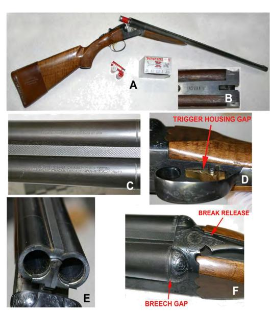
Figure 4: The shotgun. A: Full view of the Ithaca shotgun with the Winchester- ame Load box and cartridges used in the test of the shotgun. B: The serial number of the shotgun. C: Identification information on the barrels of the shotgun. D: The trigger area of the shotgun. The trigger housing gap is indicated. E: The opened breech of the shotgun. F: The closed breech area of the shotgun.
