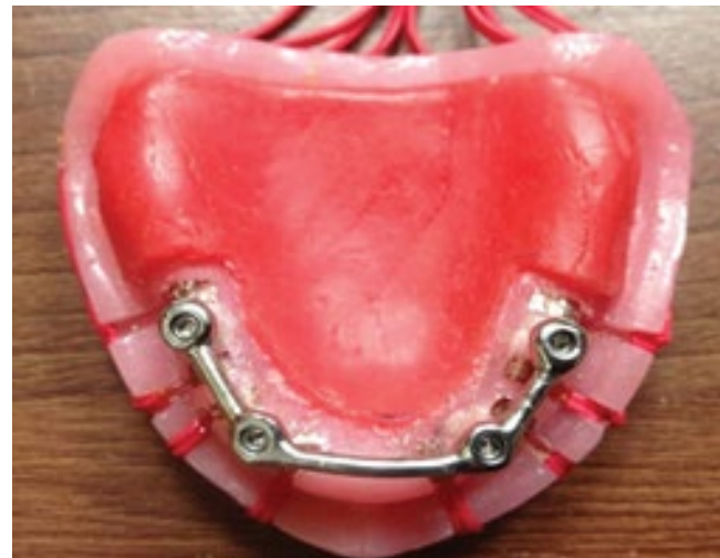
Figure 6: New strain gauges bonded to the implant fixtures.
