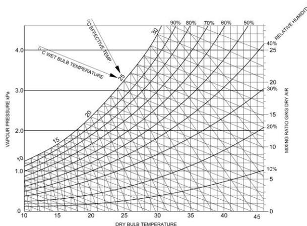
**Fig.10.** Psychrometric diagram with effective temperatur.
