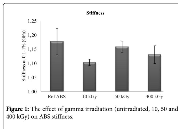
Figure 1: The effect of gamma irradiation (unirradiated, 10, 50 and 400 kGy) on ABS stiffness.
