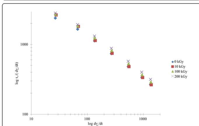
**Figure 8:** Summary of the viscosities for unirradiator ABS, 10, 100 and 200 kGy gamma irradiated ABS.
