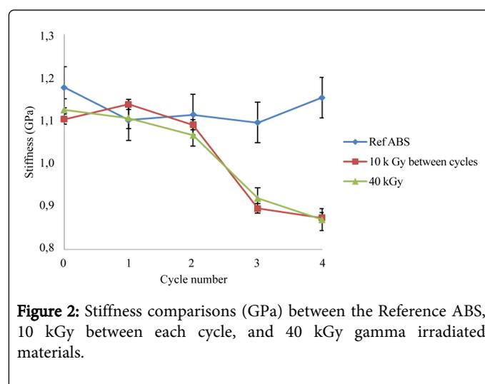
Figure 2: Stiffness comparisons (GPa) between the Reference ABS, 10 kGy between each cycle, and 40 kGy gamma irradiated materials.
