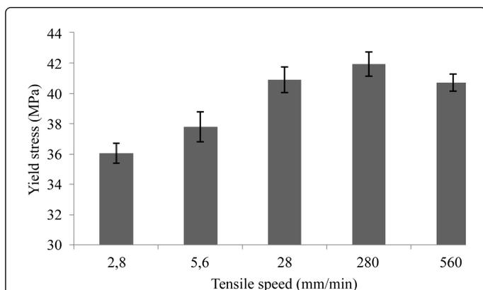
**Figure 7:** The effect of tensile speed (mm/min) on yield stress (MPa) for ABS.
