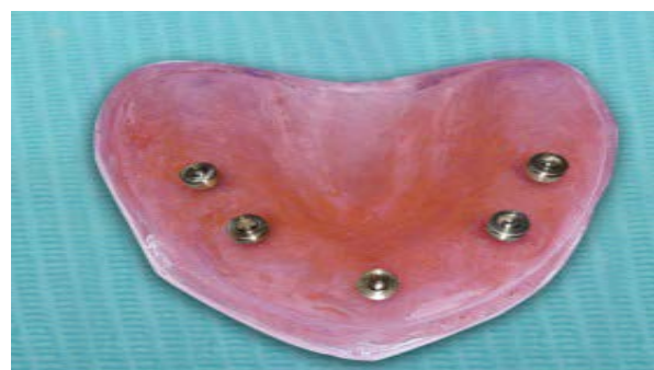
Figure 2: Heat cured polymethylmethacrylate edentulous maxillary models with V-shaped palatal vault with the dummy mini-dental implants placed parallel to each other and with O-ring.
