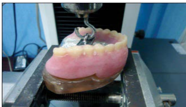
Figure 5: The simulation models were secured on the horizontal table of A Universal testing machine.
