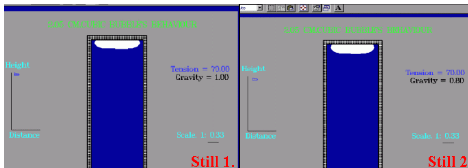
Figure 1: Gas bubble with volume of 2.05 cm 3 behavior under decreased gravity from 1 g (Still 1) consecutively to 0.8 g (Still 2).
