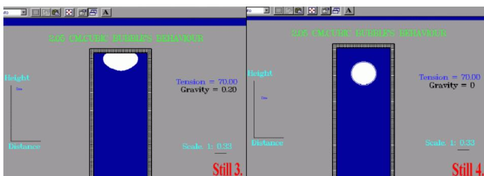
Figure 2: Gas bubble with volume of 2.05 cm<sup>3</sup> behavior under decreased gravity from 0.2 g (Still 3) and its tear from solid surface and moving down to the liquid bottom under decrease gravity from 0.2 g to g=0 (Still 4).
