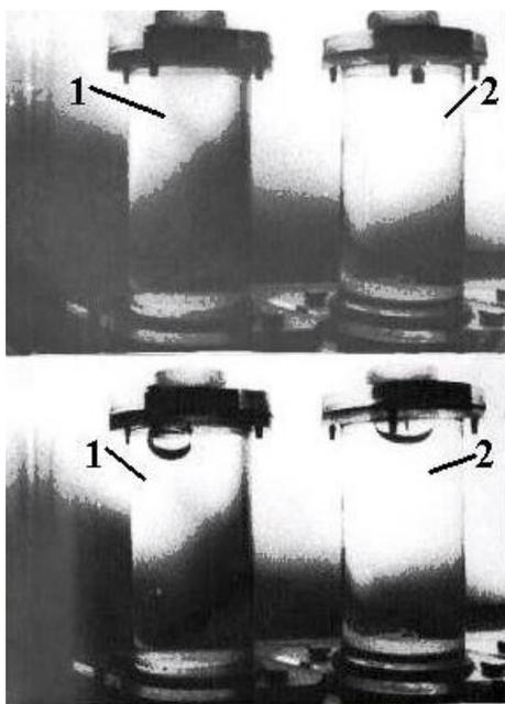
Figure 6: Gas bubbles with volume of 2.05 cm<sup>3</sup> (1) and 2.8 cm<sup>3</sup> (2) behavior under decrease gravity from 1 g to 0.2 g.
