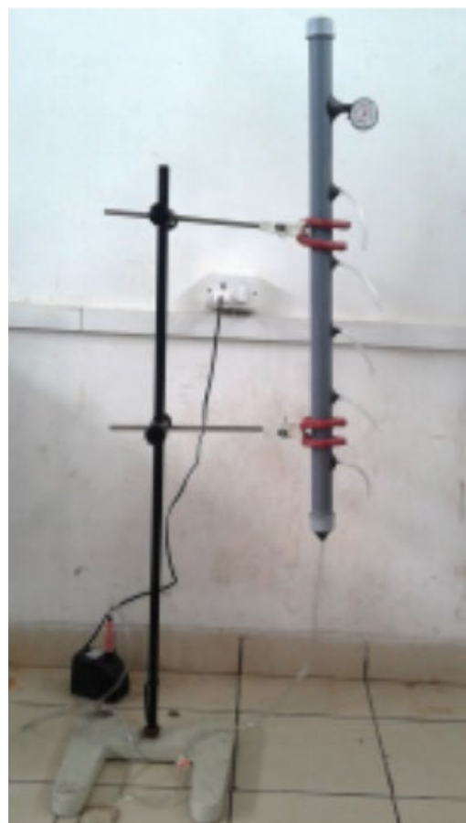
Figure 1: Experimental setup of Continuous flow column.
