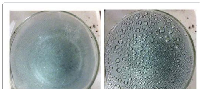
Figure 1: Nucleation of water drops on a cold watch glass; left panel early on during the process, the droplets are all small and nearly equal in size; right panel later a few large drops form as more and more water molecules get preferentially attached to the larger surfaces of the bigger drops.
