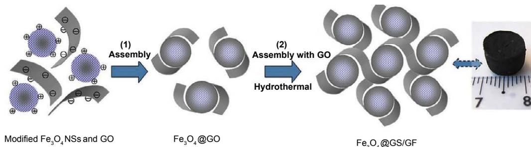
**Figure 3:** Fabrication process and photograph of  $\text{Fe}_3\text{O}_4/\text{GS}/\text{GF}$ . 1) Assembly of positively charged  $\text{Fe}_3\text{O}_4/\text{NS}$  and negatively-charged GO via electrostatic interactions. 2) Hydrothermal self-assembly of  $\text{Fe}_3\text{O}_4/\text{GO}$  and GO [26].
