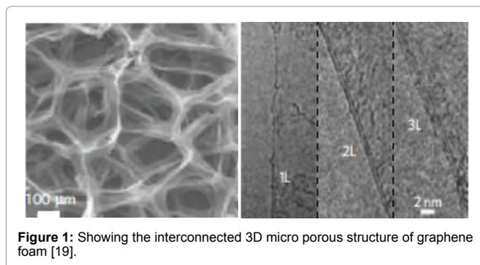
Figure 1: Showing the interconnected 3D micro porous structure of graphene foam [19].
