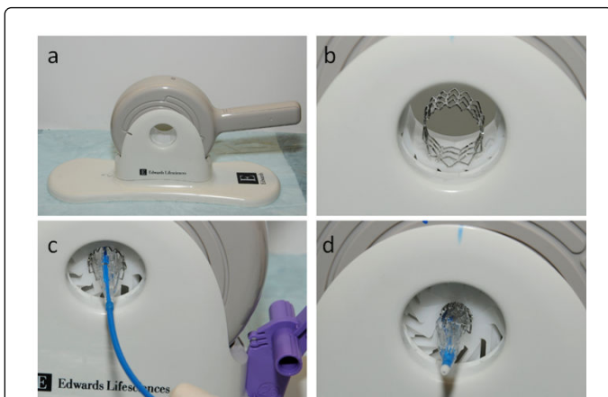
Figure 2: Disposable crimping tool holding a compression mechanism used to crimp a stent from an explanted valve Sapien XT. The stent was fitted over a balloon and was exposed to radial compression to permit its insertion within a sheath. After the crimping is completed, the mechanism is released and the stent fitted over with the balloon is pulled out.
