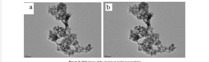
Figure 3: TEM image of the aluminum metal nanoparticles.
