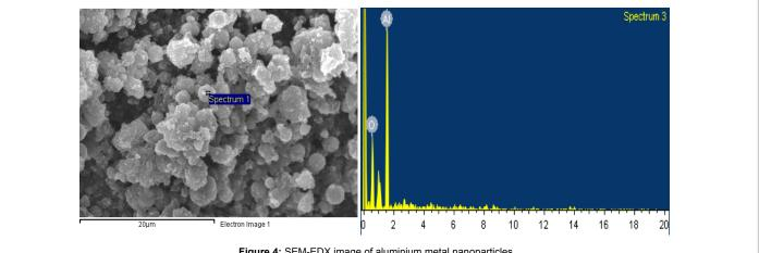
Figure 4: SEM-EDX image of aluminium metal nanoparticles.
