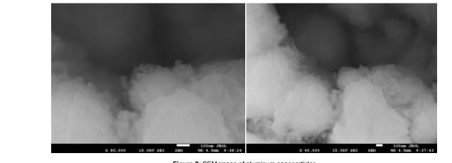
Figure 2: SEM image of aluminum nanoparticles.
