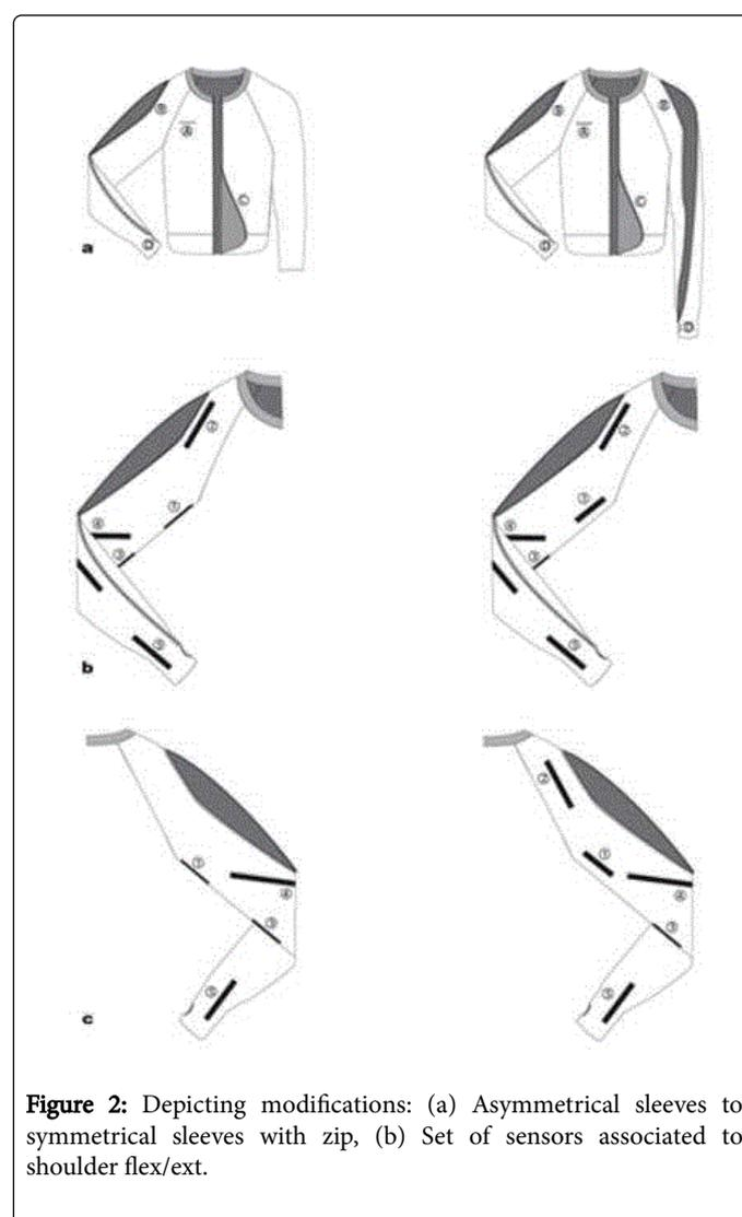
**Figure 2:** Depicting modifications: (a) Asymmetrical sleeves to symmetrical sleeves with zip, (b) Set of sensors associated to shoulder flex/ext.
