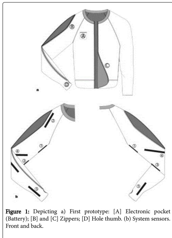
**Figure 1:** Depicting a) First prototype: [A] Electronic pocket (Battery); [B] and [C] Zippers; [D] Hole thumb. (b) System sensors. Front and back.
