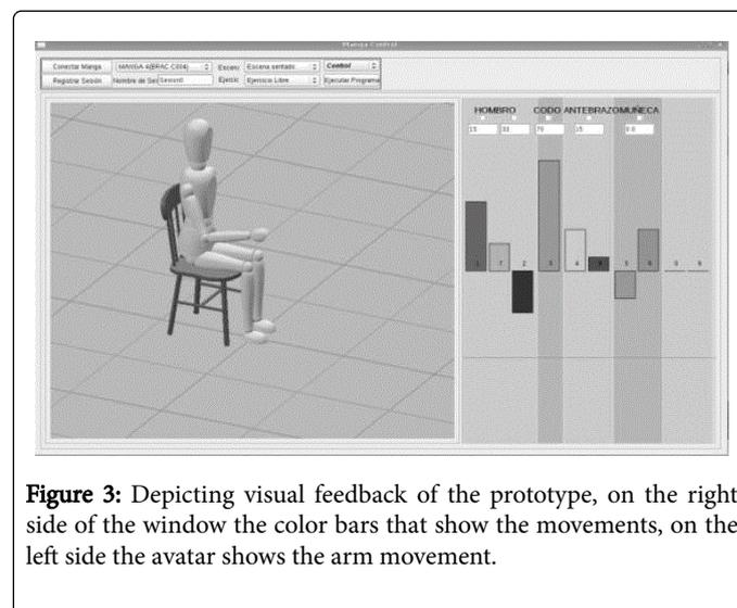
**Figure 3:** Depicting visual feedback of the prototype, on the right side of the window the color bars that show the movements, on the left side the avatar shows the arm movement.
