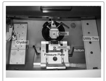
Figure 2: Test positions in the cryostat working space.
