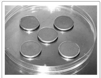
Figure 1: Virus test suspension dried onto test coupons.
