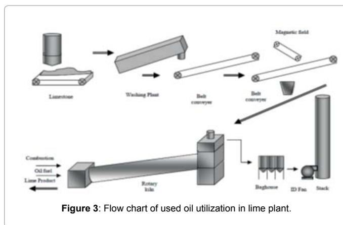
Figure 3: Flow chart of used oil utilization in lime plant.
