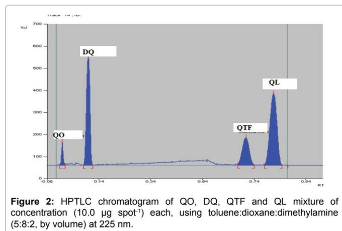
Figure 2: HPTLC chromatogram of QO, DQ, QTF and QL mixture of concentration ( $10.0 \mu\text{g spot}^{-1}$ ) each, using toluene:dioxane:dimethylamine (5:8:2, by volume) at 225 nm.
