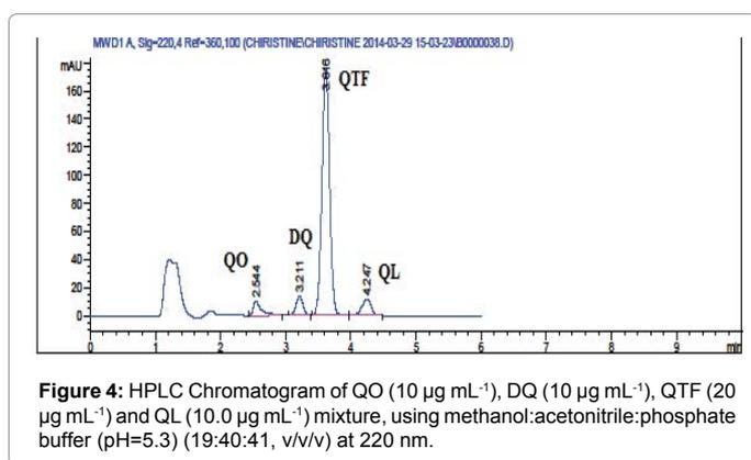
Figure 4: HPLC Chromatogram of QO ( $10 \mu\text{g mL}^{-1}$ ), DQ ( $10 \mu\text{g mL}^{-1}$ ), QTF ( $20 \mu\text{g mL}^{-1}$ ) and QL ( $10.0 \mu\text{g mL}^{-1}$ ) mixture, using methanol:acetonitrile:phosphate buffer (pH=5.3) (19:40:41, v/v/v) at 220 nm.
