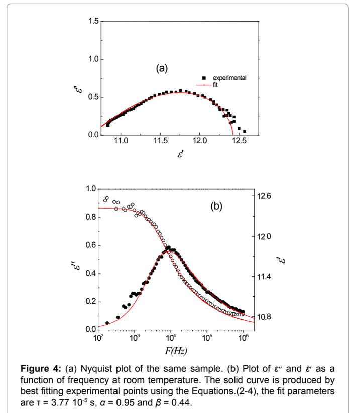
**Figure 4:** (a) Nyquist plot of the same sample. (b) Plot of  $\epsilon''$  and  $\epsilon'$  as a function of frequency at room temperature. The solid curve is produced by best fitting experimental points using the Equations.(2-4), the fit parameters are  $\tau = 3.77 \cdot 10^{-5}$  s,  $\alpha = 0.95$  and  $\beta = 0.44$ .
