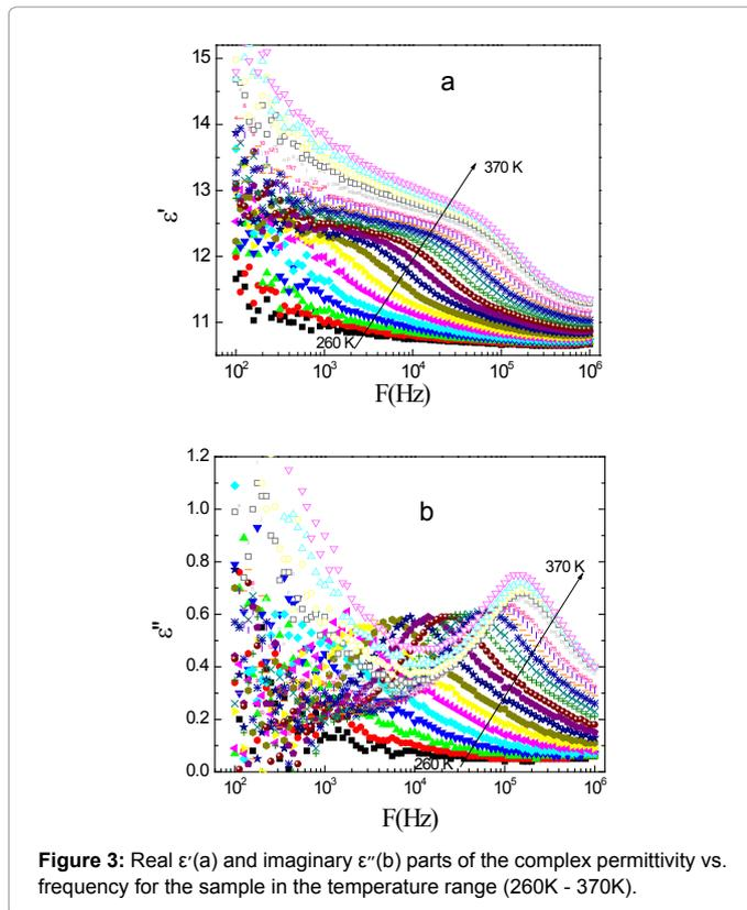
**Figure 3:** Real  $\epsilon'$ (a) and imaginary  $\epsilon''$ (b) parts of the complex permittivity vs. frequency for the sample in the temperature range (260K - 370K).
