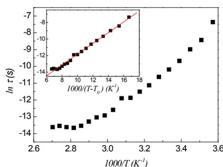
**Figure 6:**  $\ln(\tau)$  vs.  $1/T$  and the insert represents  $\ln(\tau)$  vs.  $1/(T-T_0)$ .  $T_0$  is adjustable parameter. The symbol represents the experimental data points and the solid line is the least square linear fit to VTF equation.
