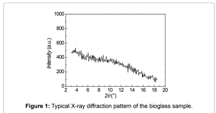
Figure 1: Typical X-ray diffraction pattern of the bioglass sample.
